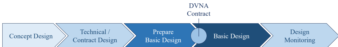
Figure 2.3: Design stages of De Voogt Naval Architects (2024)
